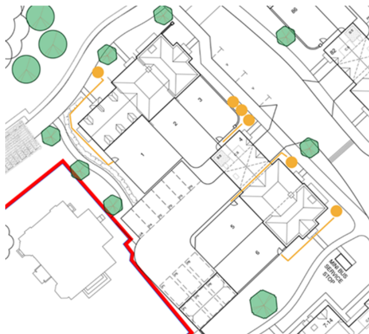
Figure 10: Refuse Storage Arrangements 1
