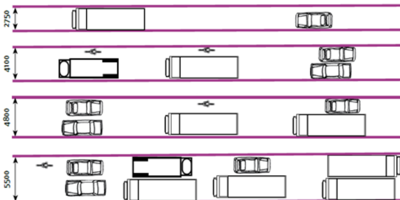
Figure 7: MfS Extract pertaining to carriageway widths
